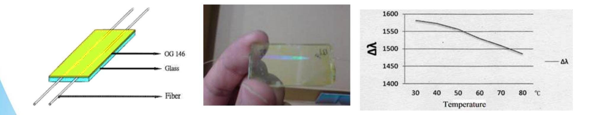
Experimental results show that, there is no change of device characteristics after the high-energy gamma-ray irradiation.
