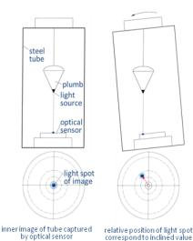
Aperture photometry modules calculates the centroid of the light spot.
